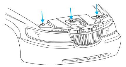
3. Twist the plastic knobs and remove the protective cover from the back of the headlamps. Lift the cover and pull towards the windshield.
